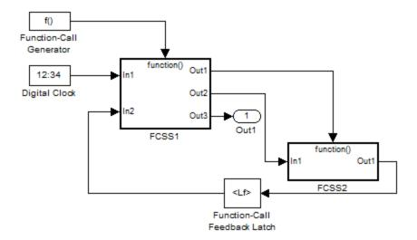
• If a loop involves function-call blocks connected to branches of the same function-call signal, then this block latches the signal at the input of the destination function-call block, and thereby allows it to execute prior to the source function-call block.
