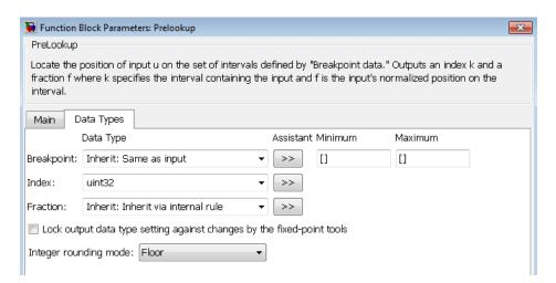
• For the Interpolation Using Prelookup block, you can now specify table, intermediate results, and output attributes on a single tab.
