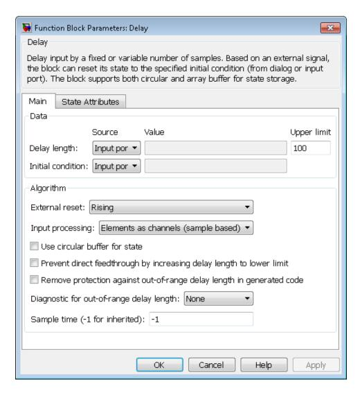
When you open models created in previous releases, the new Delay block replaces each instance of the Integer Delay block, which no longer appears in the Discrete library. The Delay block is an upgrade of the Integer Delay block. Every parameter from the Integer Delay block maps directly to a parameter in the Delay block.
