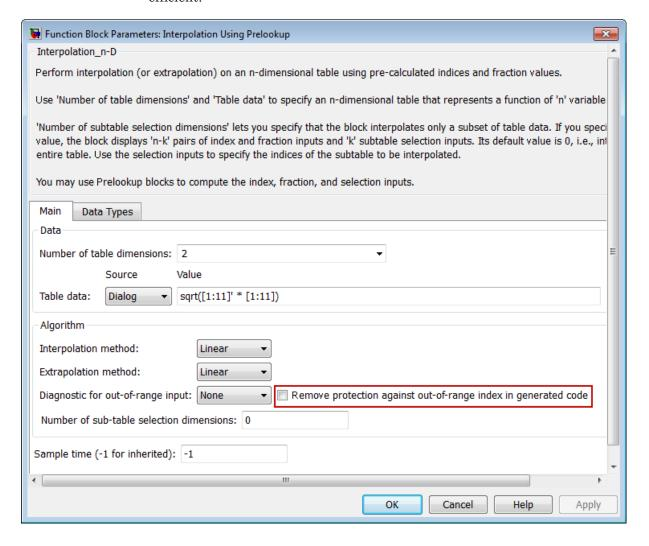
The Remove protection against out-of-range index in generated code check box replaces the Check index in generated code check box from previous releases. When you load models with the Interpolation Using Prelookup block from previous releases, the following parameter mapping applies:
