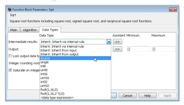
This enhancement enables explicit specification of the data type. In previous releases, specification of this data type was limited to inheritance rules.
